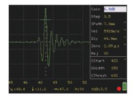
o Display original waveforms, especially suitable for R&D purpose in qualitative and spectrum analysis on echo signals.
