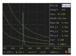
Three curves of different equivalent values will be auto created by taking a known flat-bottom hole or large flat-bottom echo for reference.
